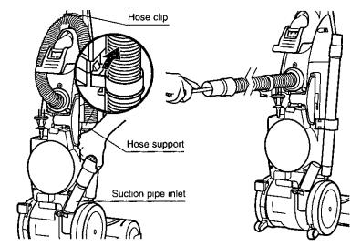
1) Remove the hose from the suction pipe inlet, hose clip and the hose support
